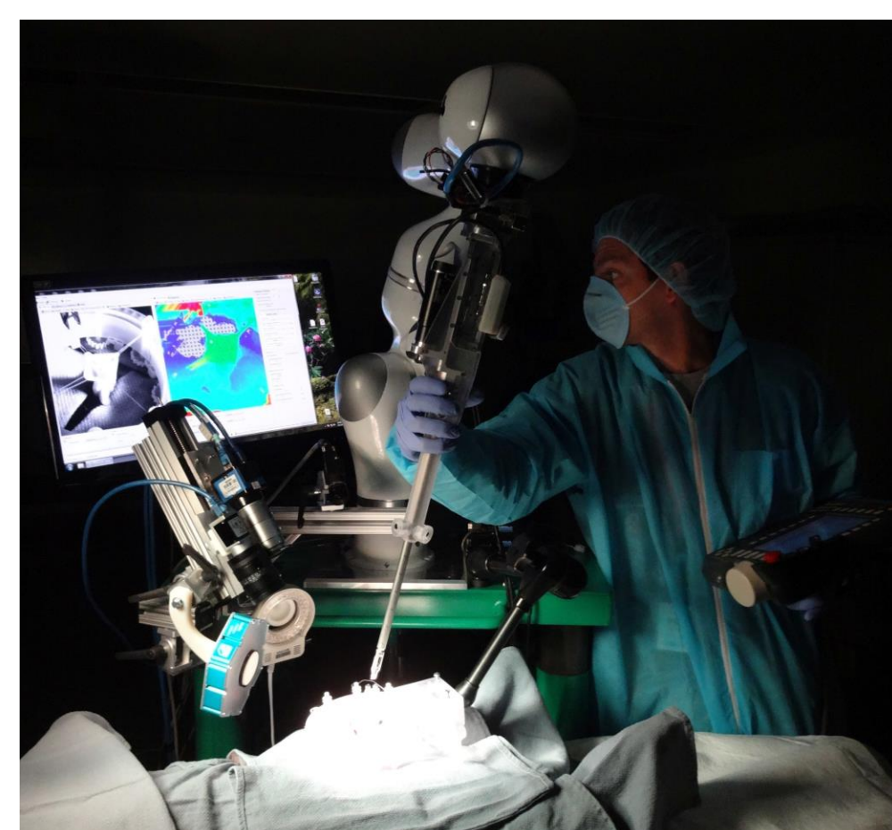
Smart Tissue Autonomous Robot (STAR), Sheikh Zayed Institute for Pediatric Surgical Innovation, Children's National Health System
