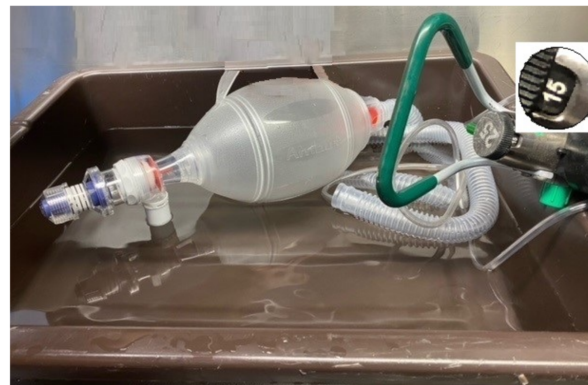
Figure 1. Self inflating bag with patient connection port submerged in water while oxygen is connected at a flow rate of 15L/min with PEEP valve. Lack of bubbles in the water demonstrates lack of forward flow through the system.
