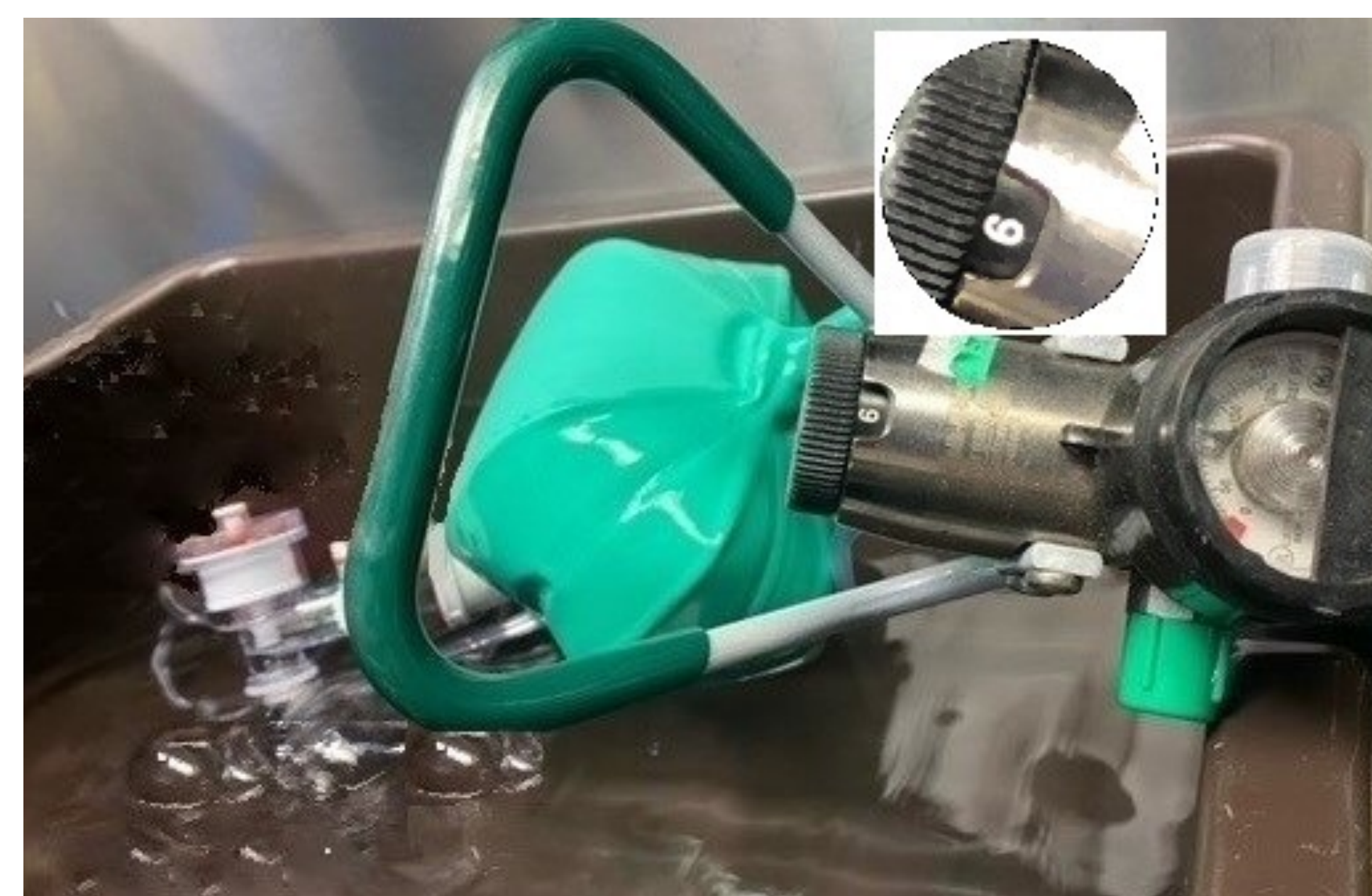
Figure 2. Flow inflating bag with patient connection port submerged in water while oxygen is connected at a flow rate of 6L/min. Bubbles in the water demonstrate presence of forward flow through the system.
